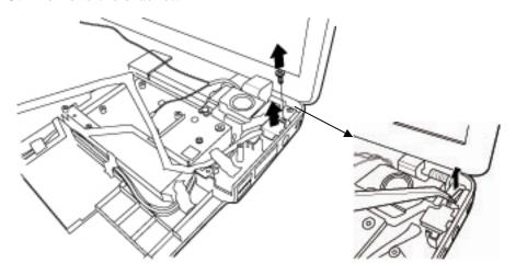
Figure 4-32 Removing screw securing bracket
